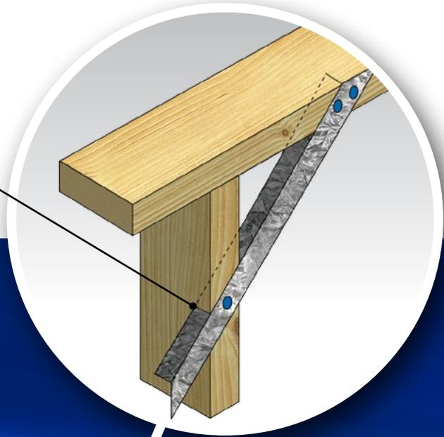
MiniBrace fixed with 1 MiTek nail to each stud and 2 MiTek nails to each wall plate
