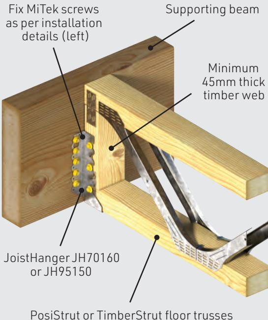
PosiStrut or TimberStrut floor trusses
